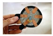
Instead of treating each conductive petrof the this fabric tilt sensor as an individual input, the petals are connected resistive fabric ring. The end petals in t "resistor ladder" connectto GND and VC create a voltage divider (just like inside potentiometer) and the bead makes for [...]
