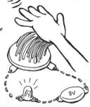
Thread the needle with conductive thread, feel free to take the thread double or quadruple. Stitch into the neoprene from the top side (the side without conductive fabric), but don't pull the thread all the way through. After stitching cut the thread at desired fur length, roughly 2cm. Repeat 5 or 6 times. Each time the conductive thread should penetrate all the way through the neoprene and make contact with the conductive fabric fused to the reverse side.
