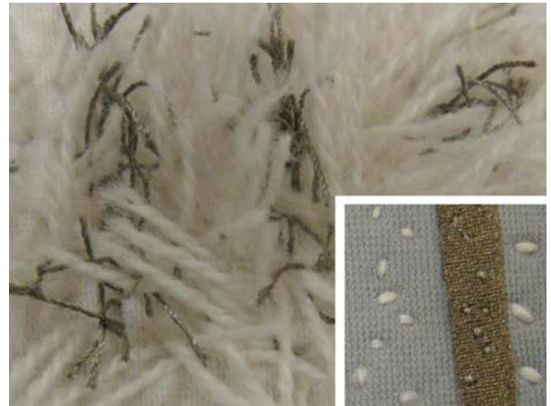
Figure 11. Stroke Sensor front, variation c, with non-conductive wool, close-up of reverse
