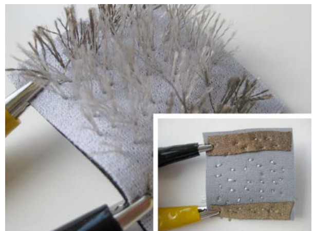
Figure 12. Stroke Sensor front, variation c, with resistive thread, close-up of reverse
