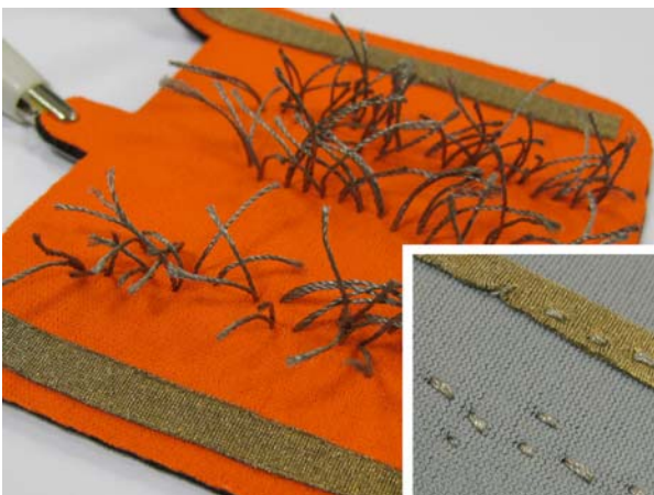
Figure 10. Stroke Sensor, variation b, two directions, close-up of reverse
