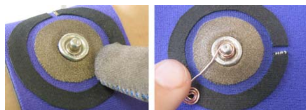
Figure 5. Fabric Potentiometer with finger cap and rotating wire hand
