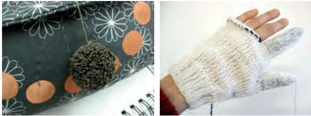
Figures 9) Participant projects: Conductive fabric pompom on purse (left), Knit glove stretch sensor (right).
