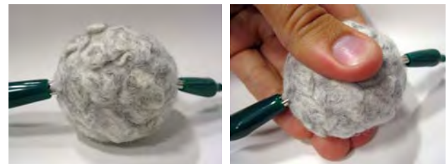
Figures 3) Felted pompom pressure sensor with alligator clips connected to either side.
