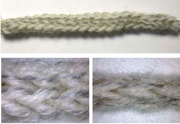
Figure 4) Tubular knit stretch sensor (top), close-up views of relaxed (bottom left) and stretched (bottom right) states.
