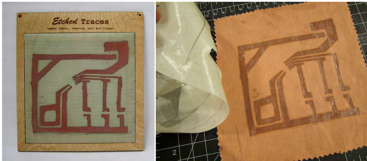
Figure 51. Etched Traces. Left: Example of circuit etched from copper rip-stop fabric. Right: Removing the masking tape stencil after applying Vaseline to the copper fabric as a resist.
