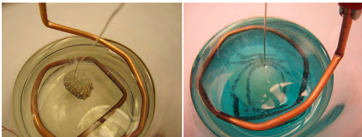
Figure 36. Left: Preparing my own etching solution from salt and vinegar. After some time the solution begins to turn light blue. Right: My own etching bath prepared by dissolving citric acid in distilled water. After awhile the solution turns blue, as the picture shows.
