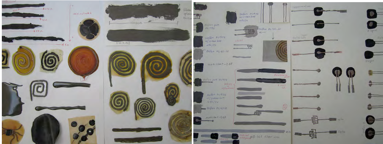
Figure 13. Left: Samples of conductive paints and powders mixed with latex in an attempt to make a stretchy conductor that can be cast. Right: Samples of conductive paints and rubbers mixed with various mediums such as matte acrylic medium, fabric medium, latex and puffy fabric paint in an attempt to create paintable substance with piezoresistive properties.
