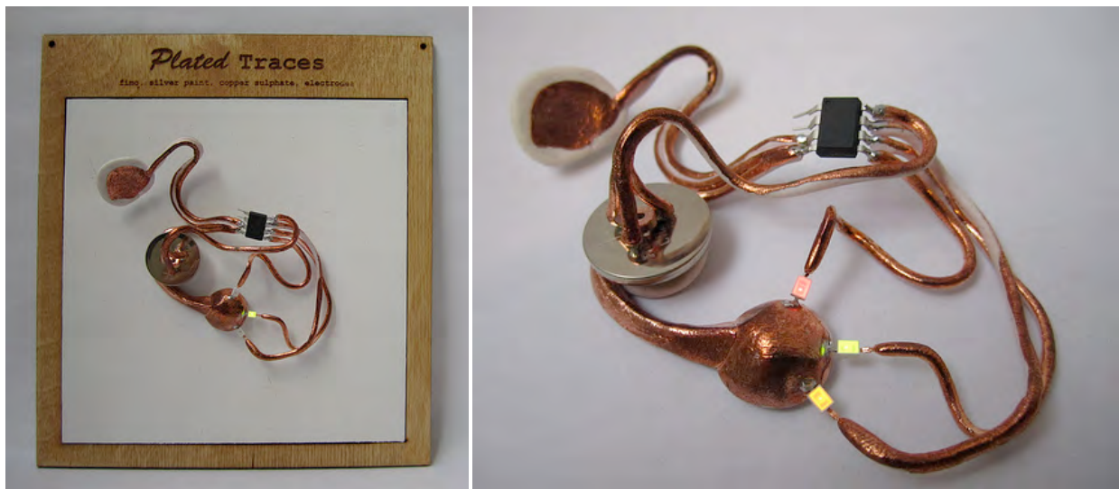
Figure 58. Plated Traces. Left: Example of plated traces as it appears in the example collection. Right: Close-up of the example with all three LED lights lit up.
