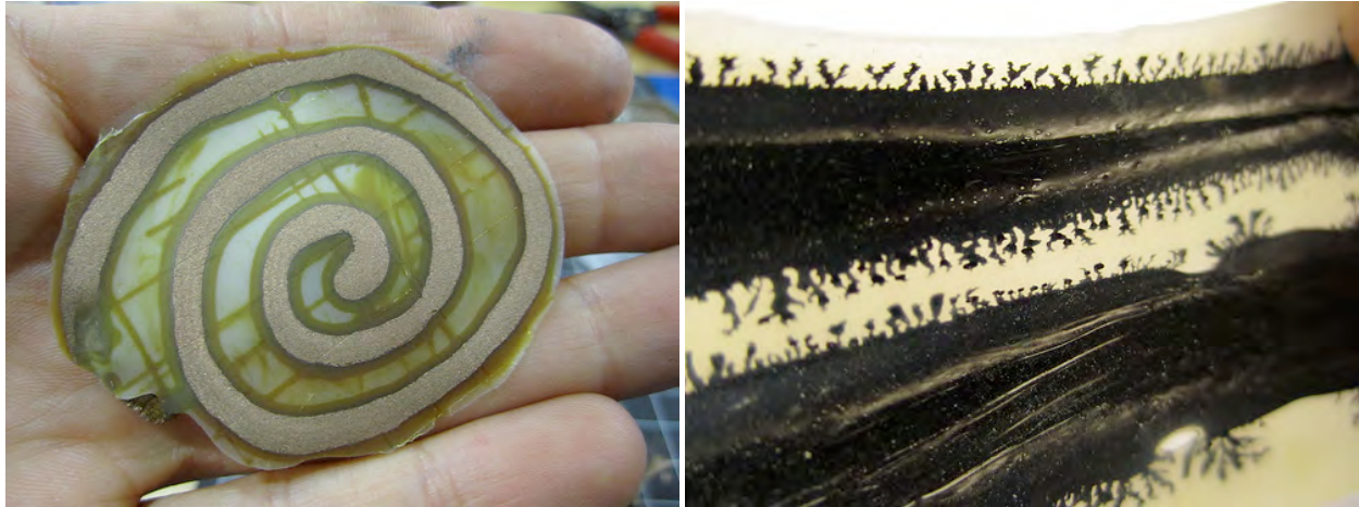
Figure 18. Left: Example of a cast speaker coil from conductive copper paint and latex. The copper particles have sunk to the bottom (side shown) of the latex, creating an isolating layer on top and exposing them on the bottom. Right: Carbon paint mixed with latex and cast in uncured latex. Not conductive but the black carbon paint trickled out into the latex at the edges creating an interesting pattern.
