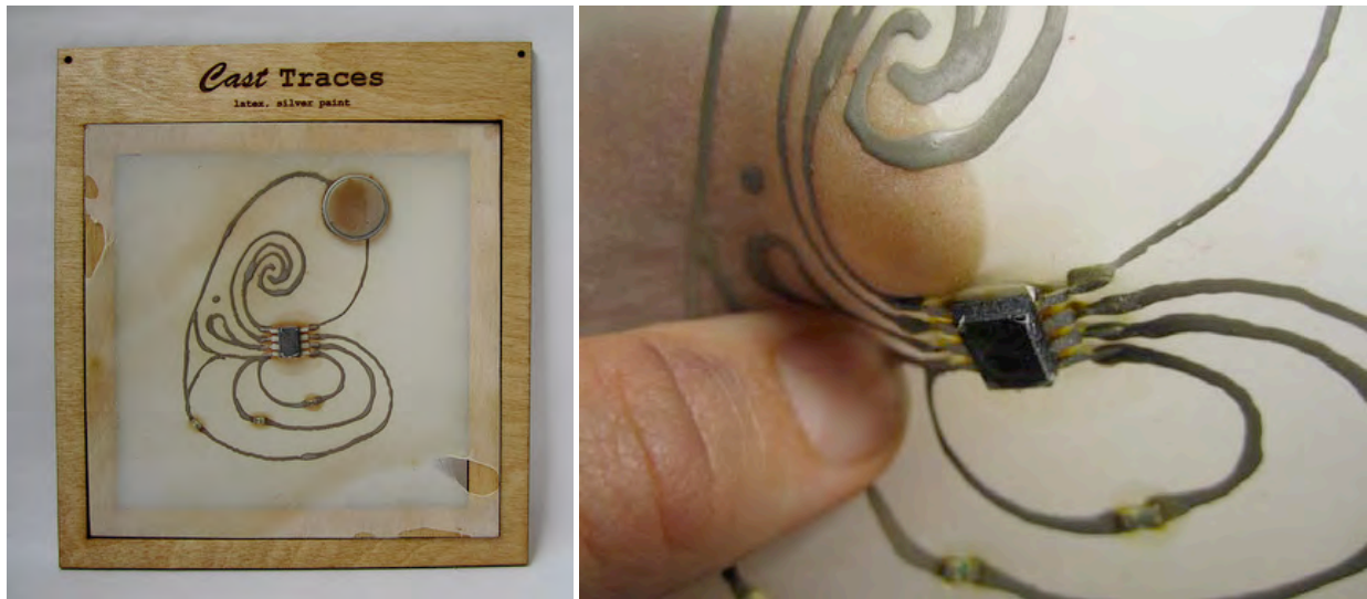
Figure 50. Cast Traces. Left: Example. Right: Close-up of microcontroller, demonstrating the stretchiness and flexibility of this circuit.
