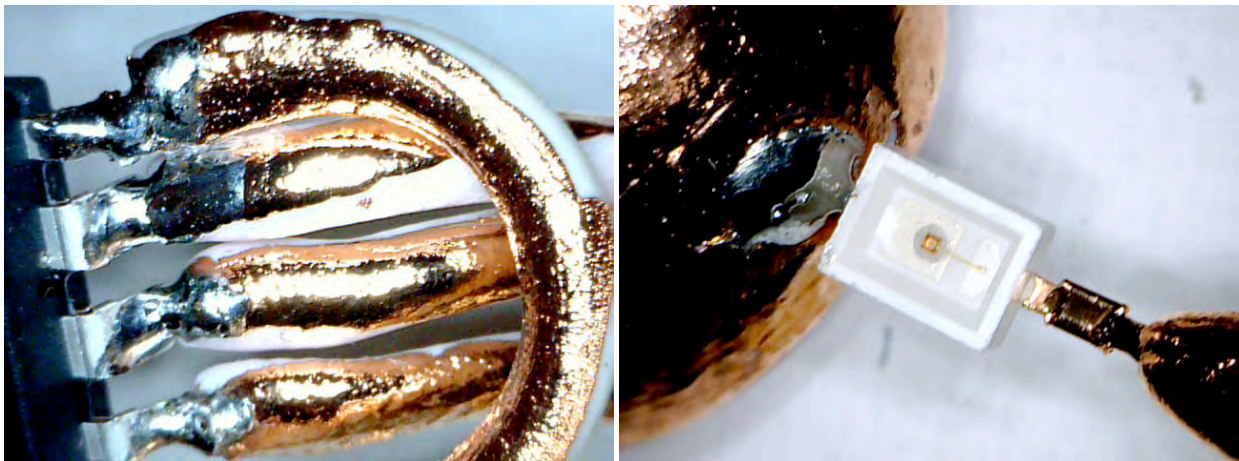
Figure 41. USB microscope images of the soldered and plated connections.
