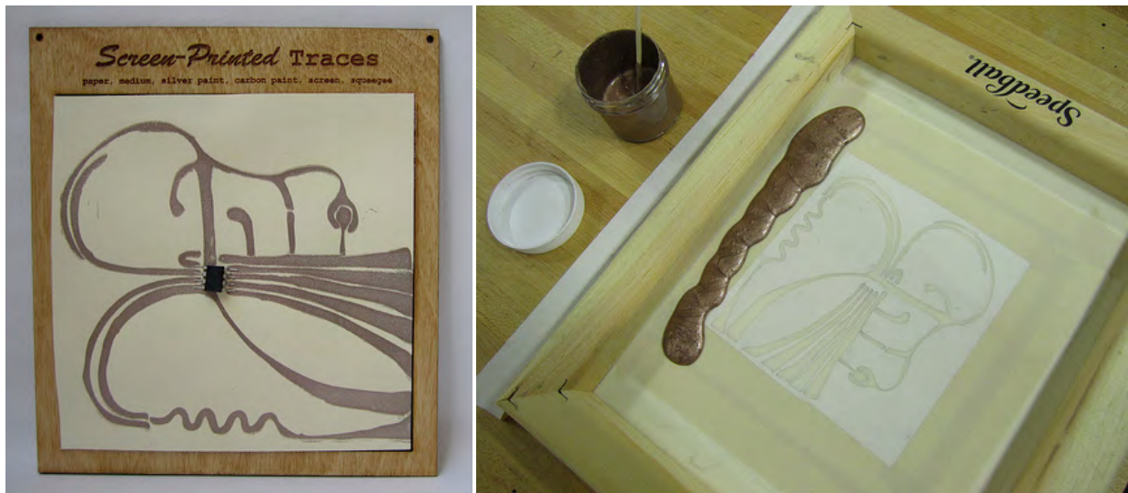
Figure 59. Screen-Printed Traces. Left: Screen printed circuit on paper. Right: Screen printing using conductive copper paint and masked silk screen.
