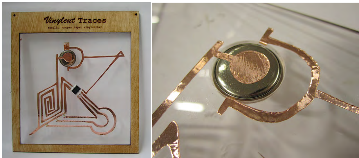
Figure 61. Vinylcut Traces. Left: Copper traces mounted on clear acrylic. Right: Press-fit hole containing coin-cell battery and copper traces making power connections to the battery along its sides and bottom.
