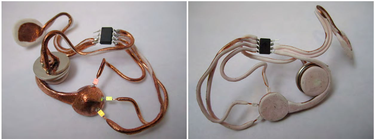
Figure 43. Images of the front (left) and back (right) of the copper plated circuit.
