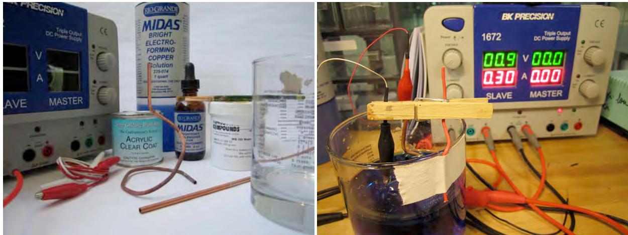
Figure 29. Left: Electroplating supplies: Rectifier, copper sulfate, replenishing brightener, copper rods, silver paint, paint brush, glass container and alligator clips. Right: Snapshot of my electroplating setup.
