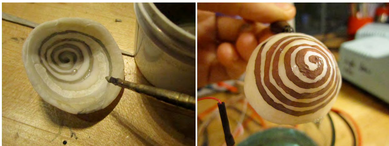
Figure 38. Left: painting seashell with conductive silver paint. Right: Seashell during plating process. After the first few seconds you can already see a fine buildup of copper.
