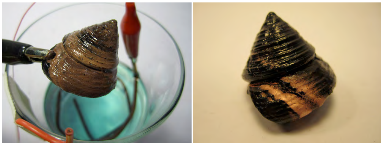
Figure 34. Plating using black carbon paint instead of silver. I did not have much luck with this. Left: Carbon painted seashell in homemade plating bath would only plate at higher voltage and copper buildup would happen fast, be contaminated and wash away. Right: Same shell after rinsing plated in commercial plating solution worked better but copper buildup would only happen in select areas, even when left in for longer periods, up to half an hour.
