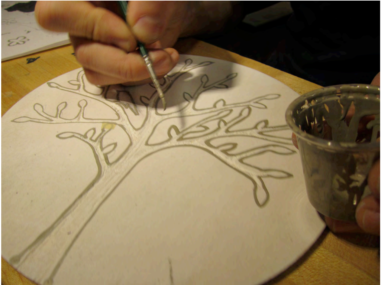
Figure 62. Picture taken during the second workshop of a participant painting a conductor that will then be used as a heating element to change the color of thermochromic paint, causing the outline of the tree to appear.
