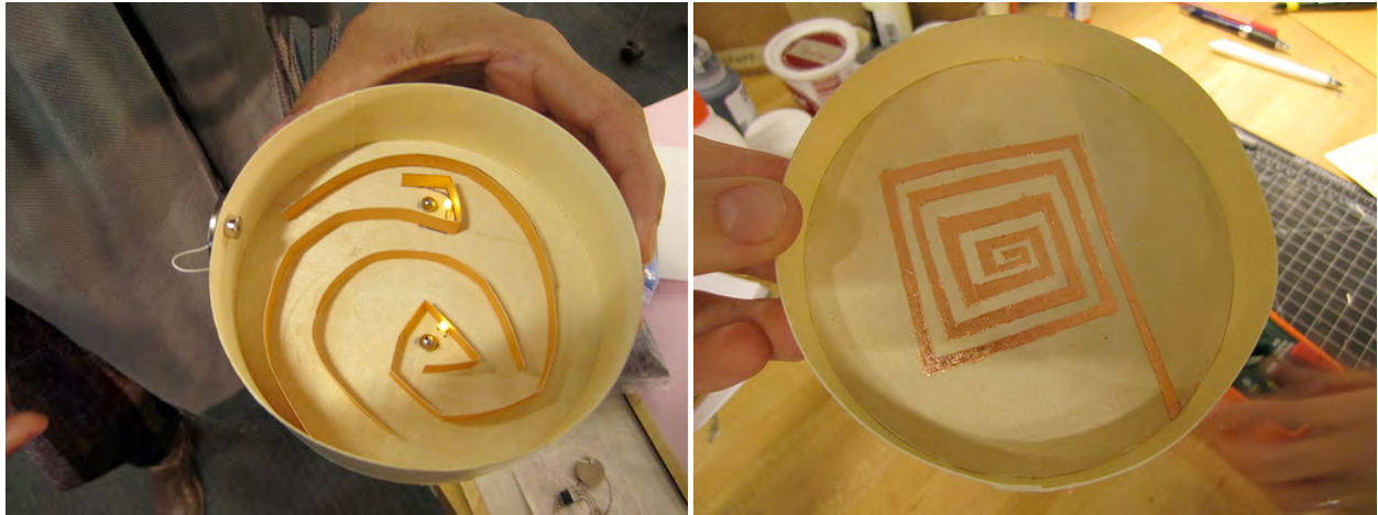
Figure 68. Left: Maze constructed inside a wooden cheese box. Right: Gilded speaker coil.
