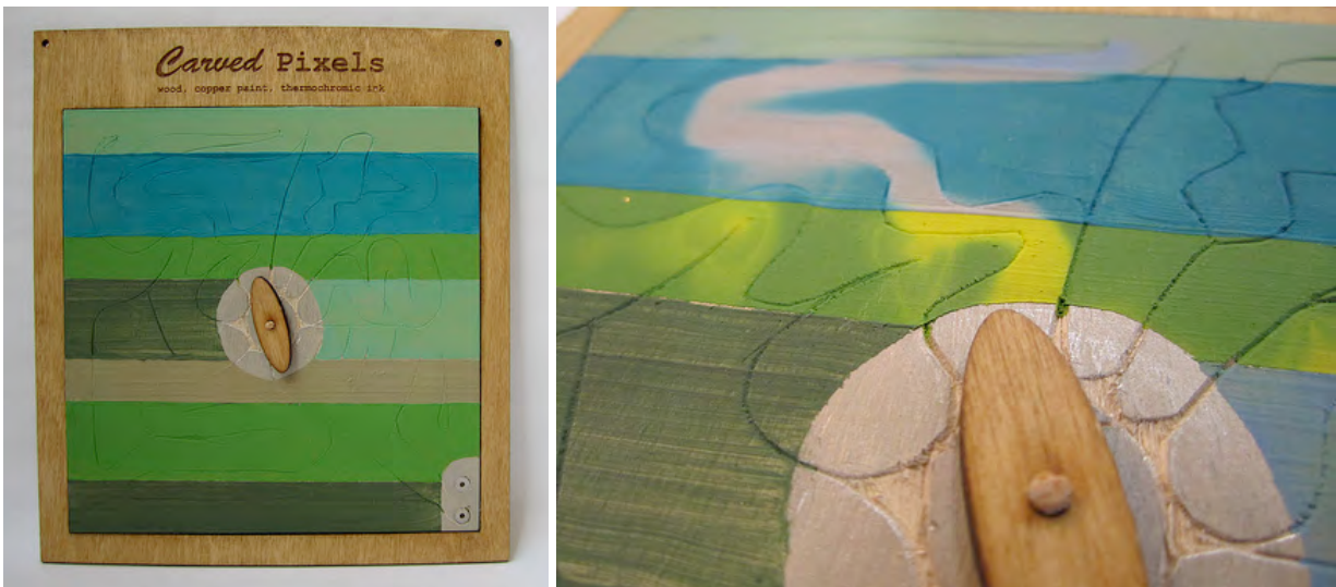
Figure 48. Thermochromic Pixels. Left: Photo of full example. Right: Close-up of dial pointing in the direction that the current is being directed. The path of the current causes the thermochromic paint to heat up and change color.
