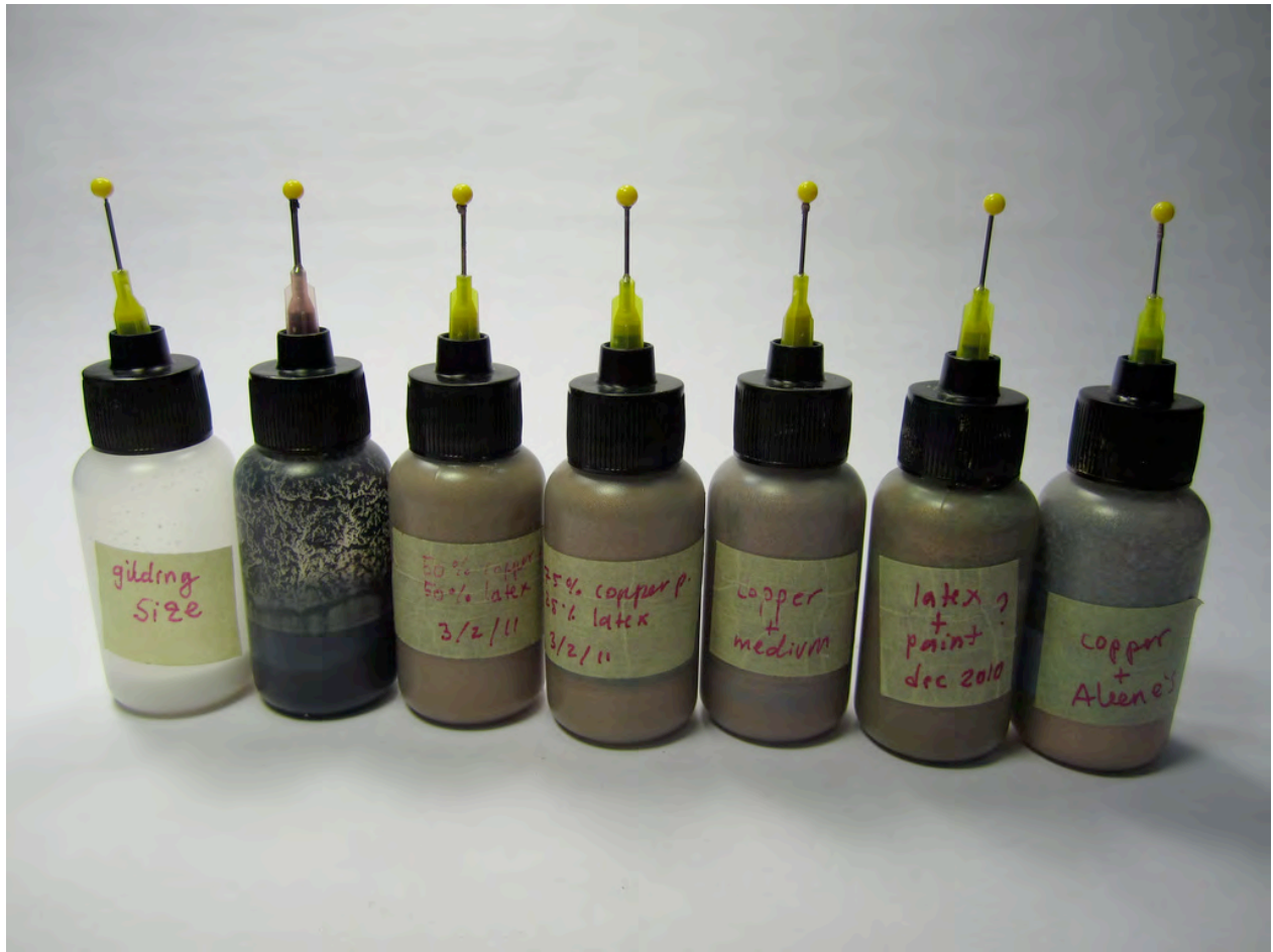
Figure 11. Collection of conductive paints mixed at different ratios, with different mediums, and stray bottle of gilding size.
