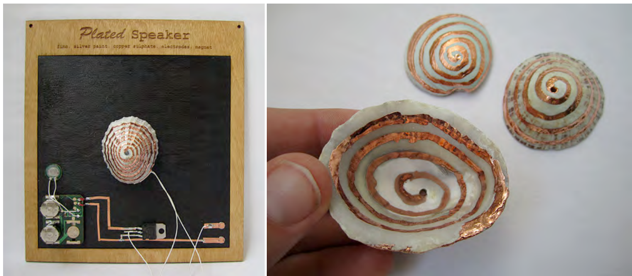
Figure 57. Plated Speaker. Left: Example of plated speaker and circuit that plays and amplifies sound. Right: Three seashells with speaker coil plated to them.
