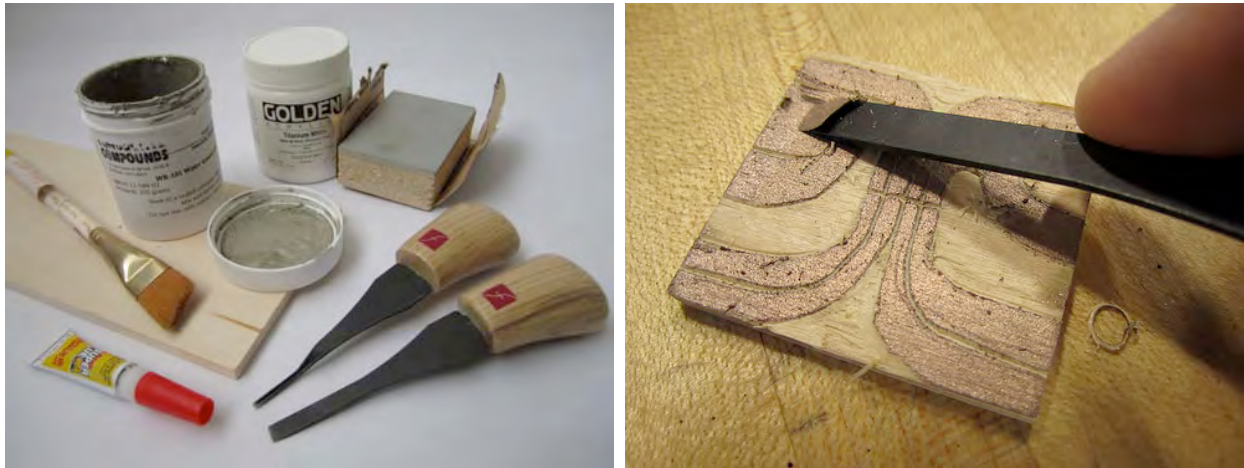
Figure 15. Left: Carving supplies. Conductive silver paint, paintbrush, wood, acrylic paint, sandpaper, carving tools and superglue. Right: Carving copper painted wood using a flat carving tool.
