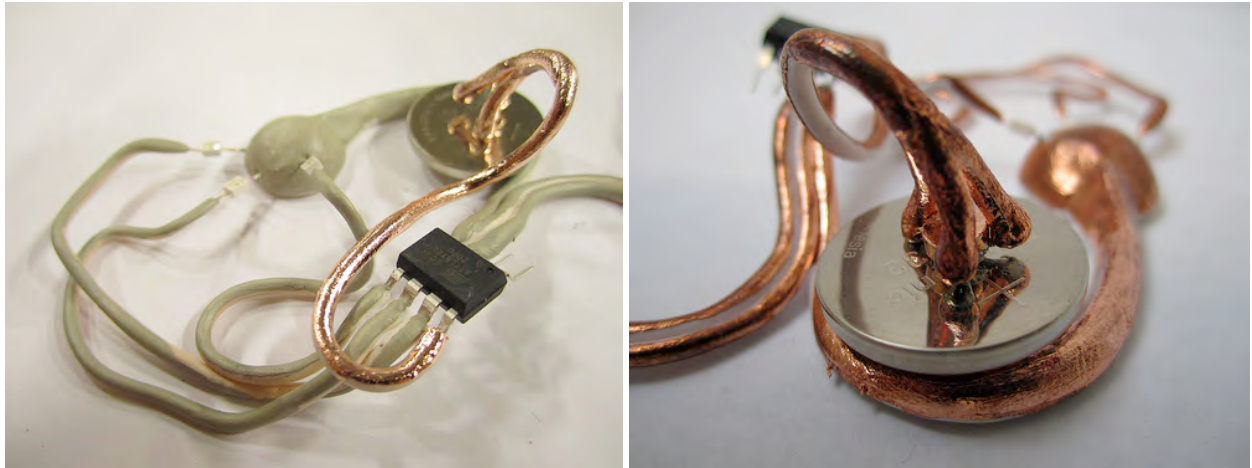
Figure 40. Left: Partially plated and assembled circuit. Right: Close-up of the magnetic battery holder.
